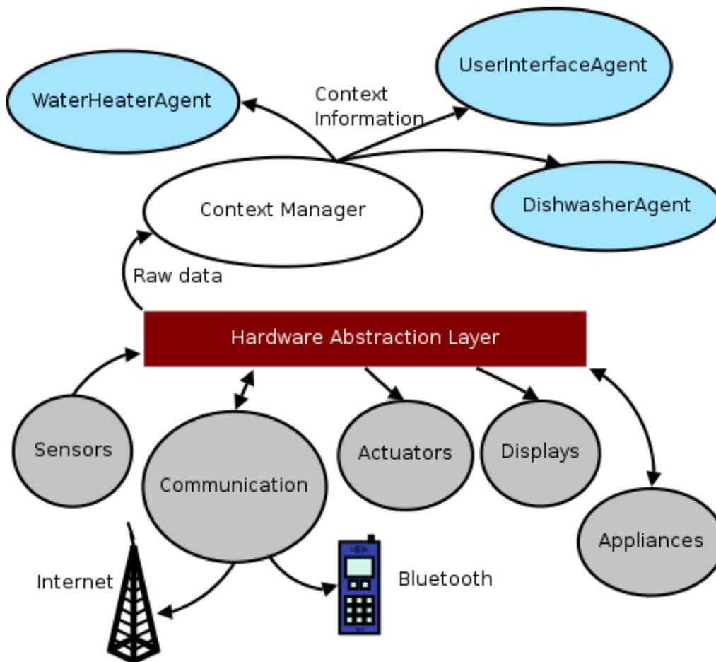
Figure 1: HAL provides the Context Manager raw data which is converted into usable context information.
